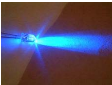
An ultraviolet GaN LED.
